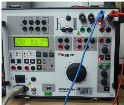
Fig. 1. Relay testing equipment SVERKER 780 at UPB laboratory.
