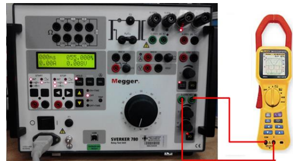
Fig. 2. Comparisons of values obtained with the SVERKER and with external measuring devices.
