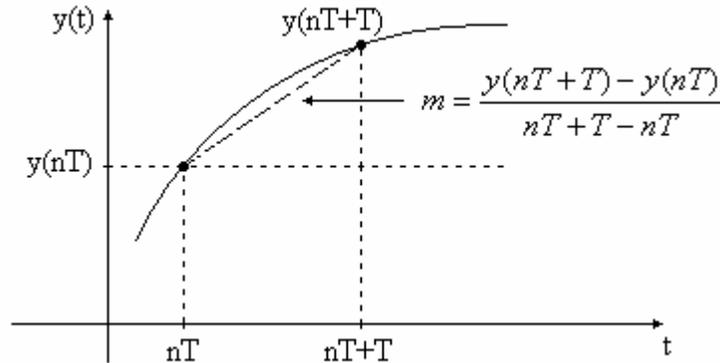
$$\left. \frac{dy}{dt} \right|_{t=nT} = \frac{y(nT-T) - y(nT)}{T}$$
