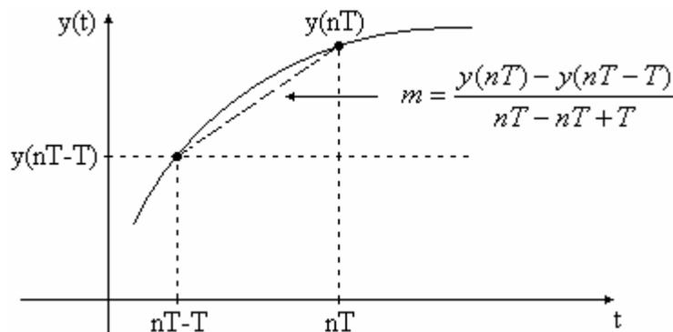
$$\left. \frac{dy}{dt} \right|_{t=nT} \approx \frac{y(nT) - y(nT-T)}{T} = -ay(nT) + bx(nT)$$
