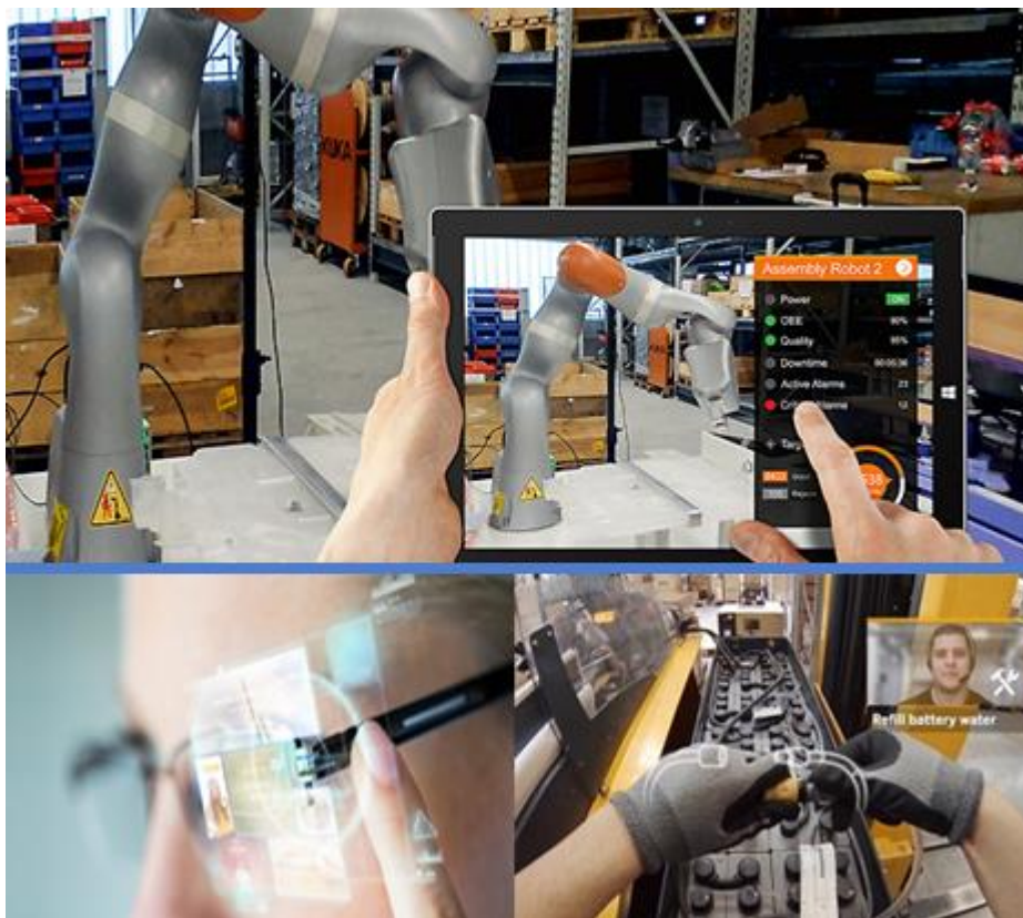
Figure 17 - An example of AR on an assembly robot(top) (Iconics Germany, 2015) and AR on a wearable(Bottom) (Critical Manufacturing, 2016; SAP, 2013)
