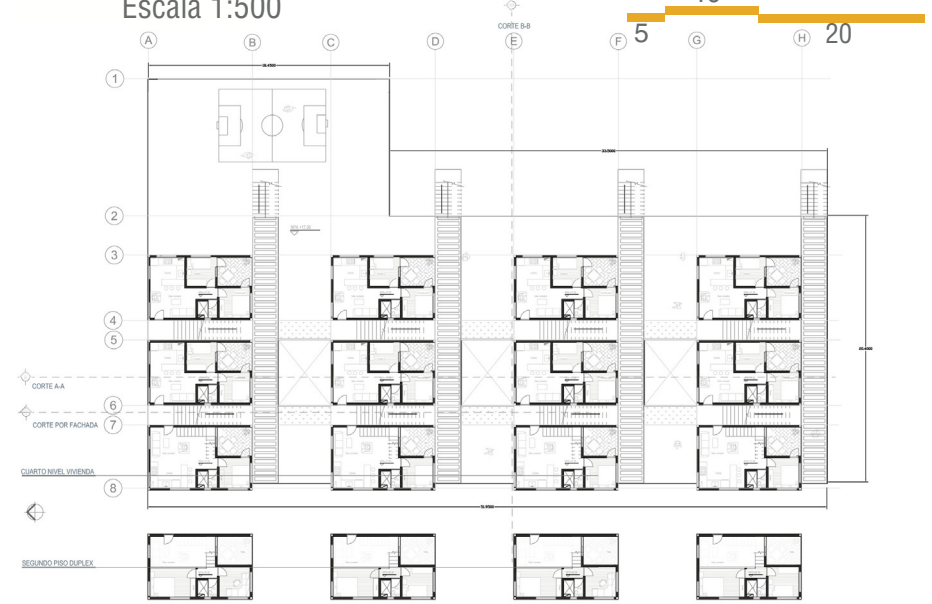
FIG 57. Planta de quinto piso/ Fifth ground floor Escala 1:500
