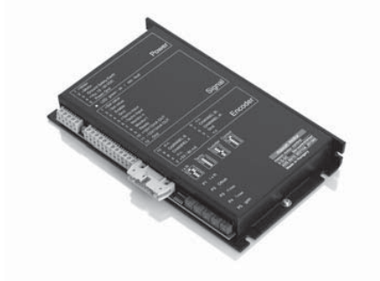
ADS 50/10 4-Q-DC Servoamplifier Powerful PWM servoamplifier for permanent magnet activated DC motors from 80 to approx. 500 watts output power. Available as Power Version in module housing.
