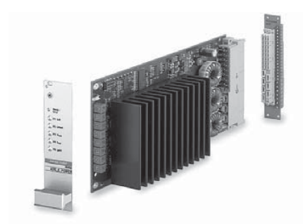
ADS_E 50/10 4-Q-DC Servoamplifier Powerful PWM servoamplifier for permanent magnet activated DC motors from 80 to approx. 500 watts output power. Available as Power Version in racket card (Eurocard) format.
