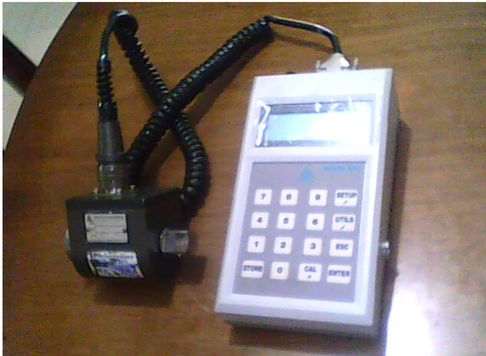
Figura 19. RS TECHNOLOGIES ROTARY TORQUE TRANSDUCER modelo No 039050-51201 junto al transductor RS TECHNOLOGIES modelo 920
