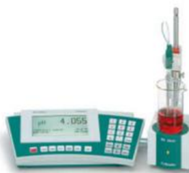
Figura 5. Phmetro - METHOHM 781 PH/ION METER.
