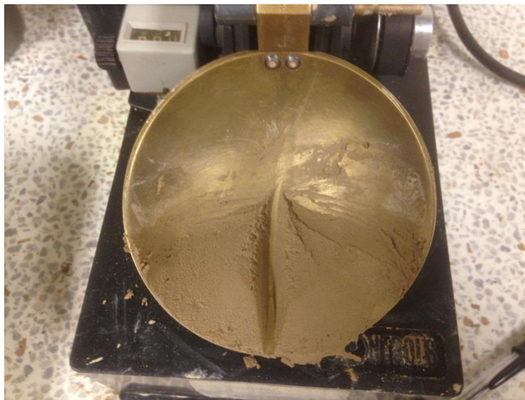
FIGURA No. 16 Limite Liquido 10% Cemento
