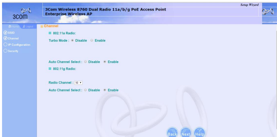
Figura 83. Interfaz Web Radio Channel del Access Point 3Com.
