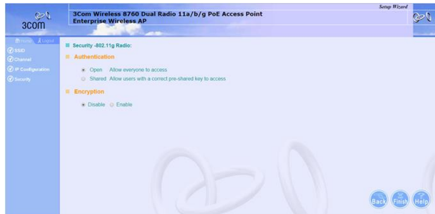
Figura 87. Interfaz Web Security 802.11g Radio del Access Point 3Com.
