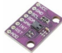
Figura 13: Sensor de CO 2 CCS811
