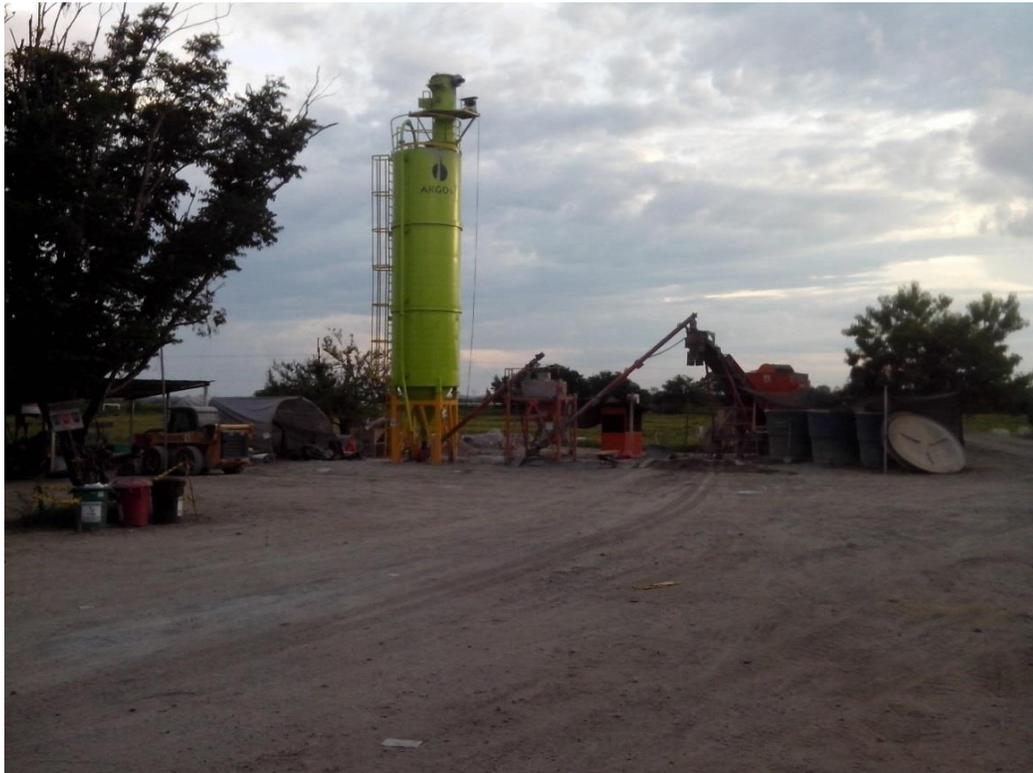
**Figura 19- Cemento a Granel- Silo Argos**
