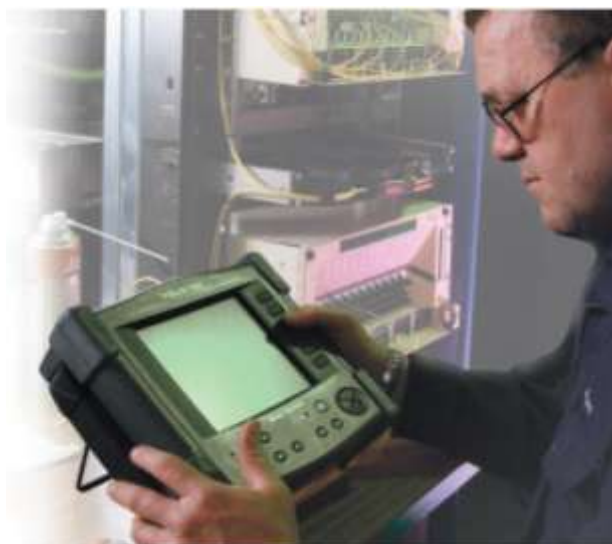
FIGURA 38. OTDR (Optical Time Domain Reflectometer):
