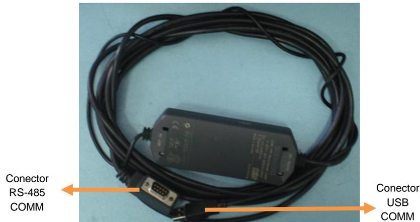
Figura 127. Cable multimaestro USB/PPI S7-200. [68]
