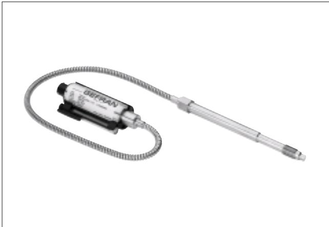
The MN series of Gefran, are pressure transmitters for using in High temperature environment. The main characteristic of this series is the capability to read temperature of the media up to 400°C. The constructive principle is based on the hydraulic transmission of the pressure. The fluid-filled system assures the temperature stability. The physical measure is transformed in a electrical measure by means the strain-gauge technology.
