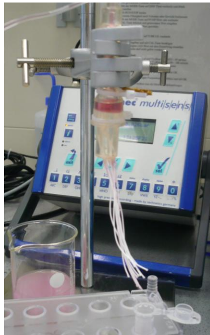
Figure 29. Half hand-bundle undergoing a dead-end GPRT.
