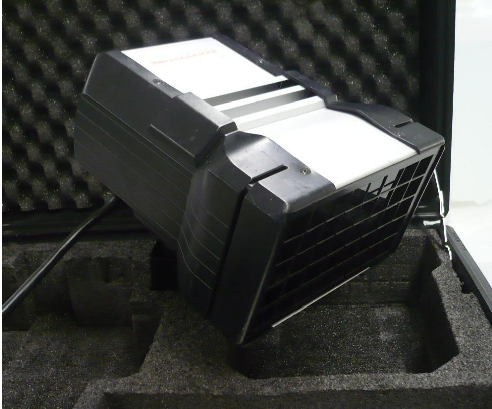
Figure 4. UV-lamp employed for the polymerization (Uvahand 250, Dr. Hönle AG, München)
