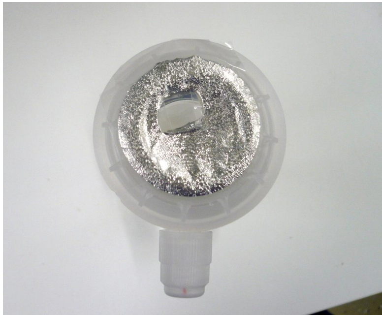
Figure 26. Reaction chamber end, sealed with aluminum-foil, the fiber moves through the opening.
