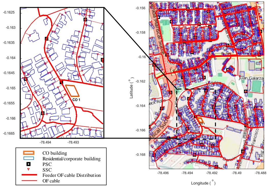
Figure 6.10: Optimal topology in a region of Quito covered by a central office (CO 1) with about 10^4 users (right figure). In the zoom at the left, it can be appreciated the detailed graphical results OTS delivers: Optimal routes for feeder and distribution OF cables, CO location and optimal location of PSC and SSC (notice in Quito’s map the SSC are also placed in the buildings while the PSC are located in the neighboring streets).
