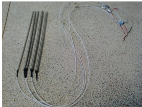
Figura 32. RTD Pt 100 (Resistance Temperature Detector)
