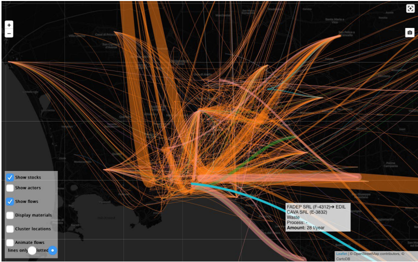
Figure 5. Activity based-material flow map of mixed construction and demolition waste (EWC 170904) produced in Naples focus area in 2015
