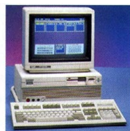
Tandy's burned MS-DOS and the Desk-Mate shell into its 1000 SL's ROM for fast bootup and anxiety-reducing ease of use.
