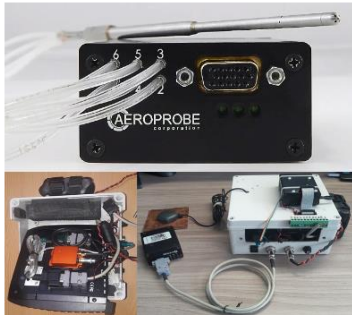
Figure 18. Instrumentation for real-time inflight state estimation.
